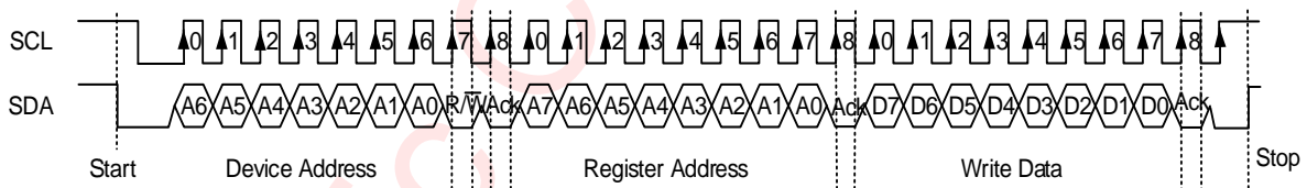
Figure 9 I 2 C Write Byte Cycle
