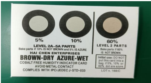
图 5-3 样品 10# 湿度指示卡 Figure 5-3. Sample 10# HIC after opening MBB
