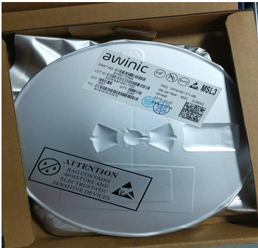
图 5-1 样品 10#打开内盒，MSL3 包装 Figure 5-1. Sample 10# Opened Box, MSL3 Packing
